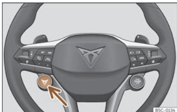
Fig. 149 Multifunction steering wheel: button to change the driving profile.
