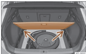
Fig. 118 Variable luggage compartment floor: inclined position.
