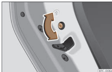
Fig. 82 Childproof lock on the left hand side door.
