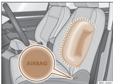
Fig. 21 Side airbag in driver's seat.
