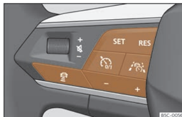
Fig. 169 Left side of the multifunction steering wheel: buttons for operating Travel Assist.
