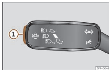
Fig. 62 On the turn signal and main beam lever: button for driver assistance systems (depending on versions).
