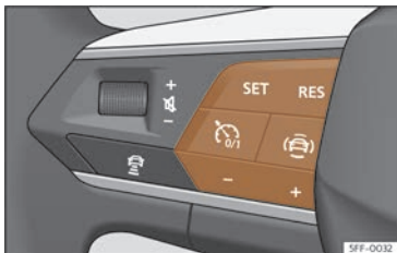
Fig. 156 On the multifunction steering wheel: buttons to operate the speed limiter.
