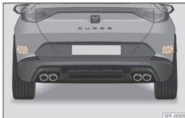
Fig. 153 Rear view of the vehicle: radar sensor zones.
