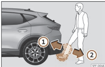
Fig. 86 Rear lid with sensor-controlled opening (Easy Open).
