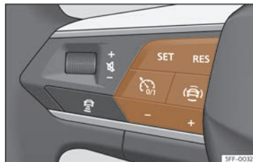
Fig. 157 On the multifunction steering wheel: buttons to operate the speed limiter.
