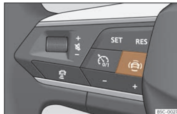
Fig. 63 Left side of the multifunction steering wheel: button for driver assistance systems (depending on versions).
