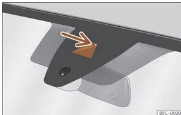
Fig. 152 On the windscreen: field of vision of the Lane Assist system.
