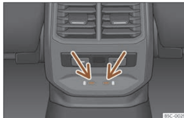
Fig. 142 Rear part of the centre console: USB connectors with power outlet function.
