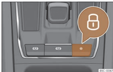
Fig. 77 In the centre console: central locking switch
