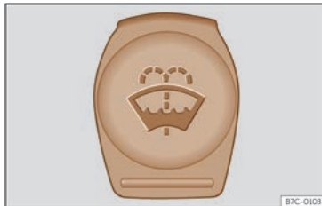
Fig. 220 In the engine compartment: blue cap of the windscreen washer tank.
