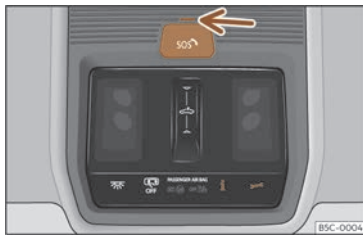
Fig. 32 On the roof console: voice service controls
