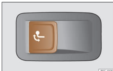
Fig. 192 On the left side of the luggage compartment: button for unlocking the tow hook.
