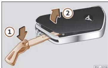
Fig. 74 Vehicle key: opening the battery compartment cover.
