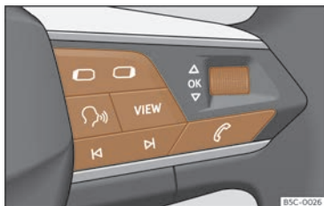
Fig. 61 Right side of the multifunction steering wheel: buttons for using the instrument cluster's menus and information displays (depending on versions).
