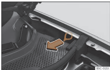
Fig. 201 Between the left wing panel and the engine bonnet hinge: Charging connector manual release mechanism puller.
