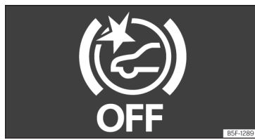
Fig. 160 On the instrument panel display: Front Assist deactivated indication.
