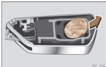
Fig. 75 Vehicle key: removing the battery.
