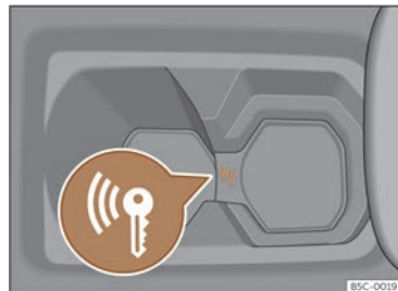
Fig. 144 In the centre console: emergency start.
