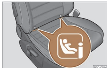
Fig. 28 Front passenger seat: ISOFIX/i-Size securing rings.
