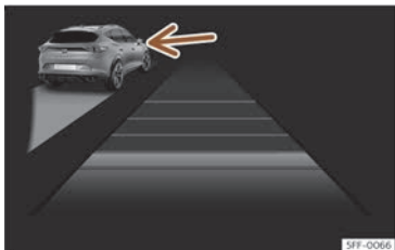
Fig. 163 On the instrument panel display: ACC active, vehicle detected in an outer lane.
