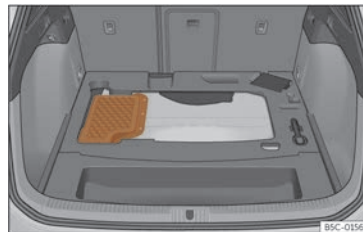
Fig. 221 Hybrid vehicles (PHEV): location of the battery in the luggage compartment
