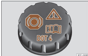
Fig. 219 Engine compartment: brake fluid reservoir cap.
