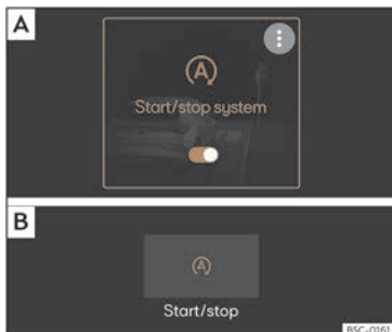
Fig. 145 On the Infotainment system screen.: Start-Stop system connected. A View in the main menu. B View with the Infotainment system off.
