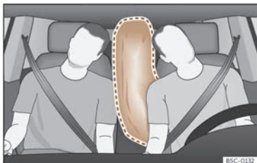
Fig. 20 Fully inflated central airbag (deployment zone).
