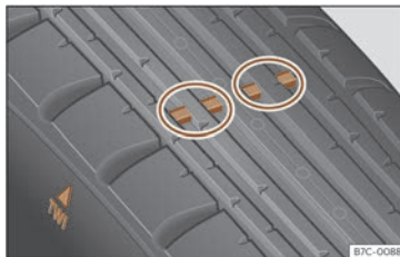
Fig. 224 Tyre profile: tread wear indicators.
