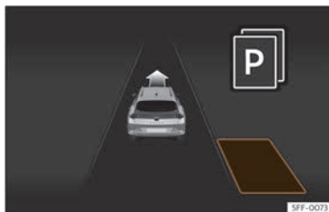
Fig. 180 On the instrument panel display: view of the parking assist system with reduced view.
