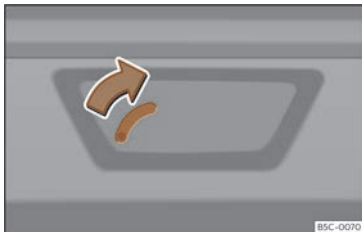
Fig. 88 Detail of the luggage compartment: emergency unlocking
